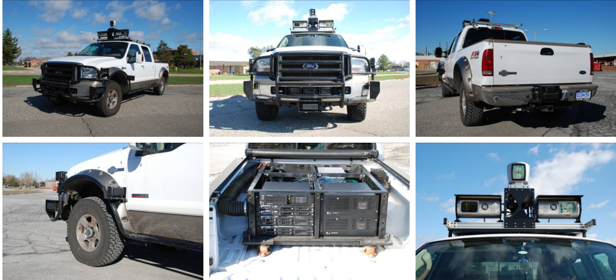
Figure 5 – Sensor placement and computer cluster on the XAV-250
