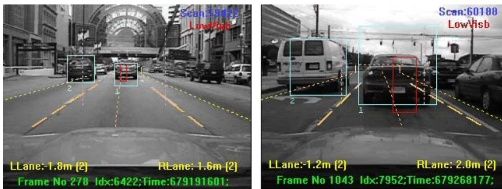
Figure 19 – Radar/Vision fusion with lane detection and closest in-path target
