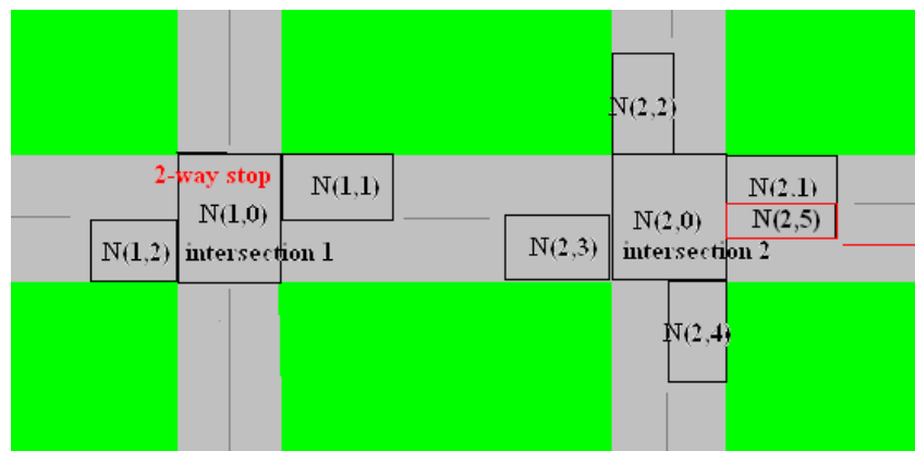
Figure 10 – Intersection Logic Details
