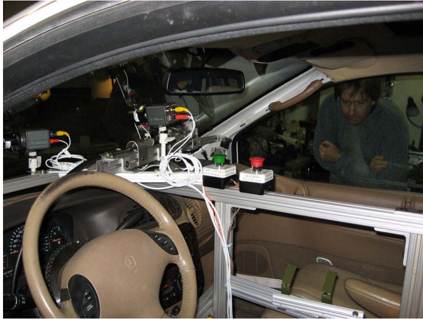
Figure 2. Steer and Brake Actuators – also shows placement of forward and side looking cameras
