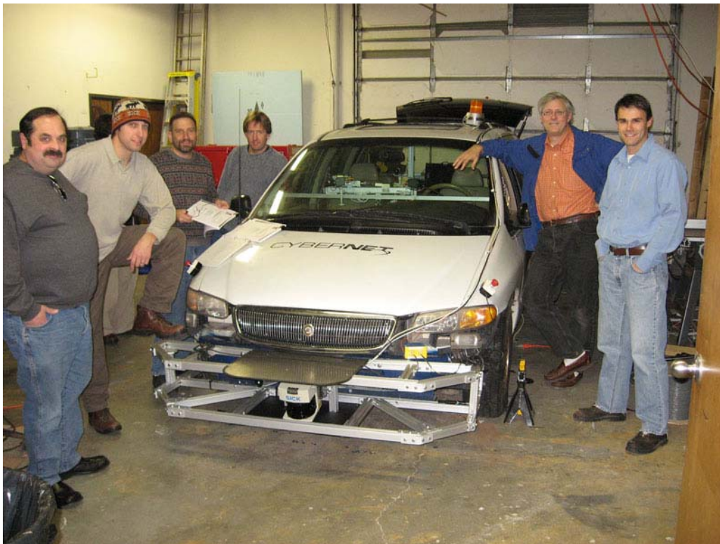
Figure 1. The Armadillo test vehicle – standard 1996 Chrysler Town & Country minivan previously used for vehicle microwave soft stopping tests 1 -- also shows forward lidar, camera and inertial measurement unit
