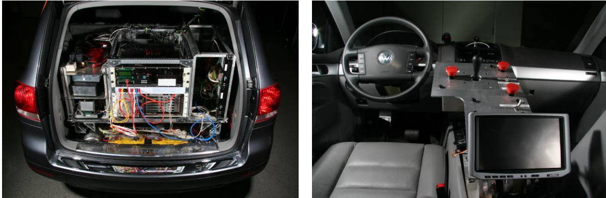
Figure A.2: Left: The computing system in the trunk of the vehicle. Right: The drive-by-wire system and the interface for manual vehicle operation.
