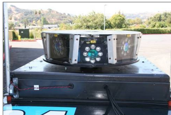
Figure 10. Rotating multiple LIDAR system from Team DAD.
