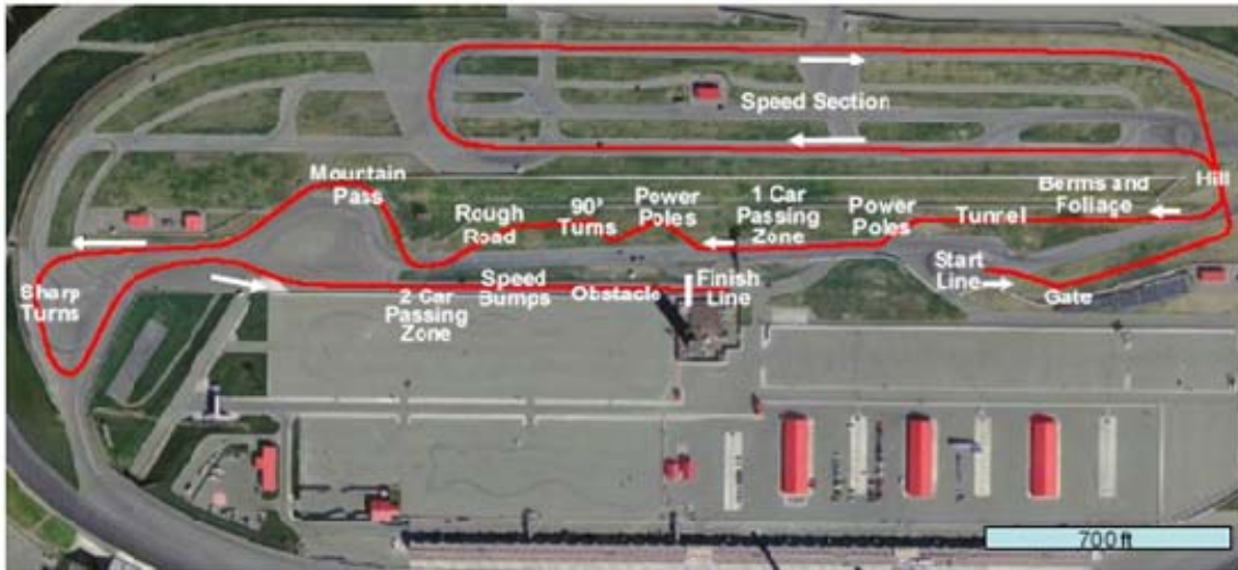
Figure 3. The NQE course layout showing the obstacles and other challenges faced by autonomous vehicles on the test course.
