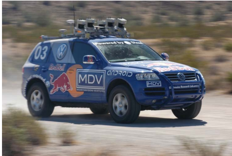
Figure A.1: Stanley is based on a 2004 Volkswagen Touareg R5 Diesel. The vehicle is equipped with a number of sensors for environment perception and localization.
