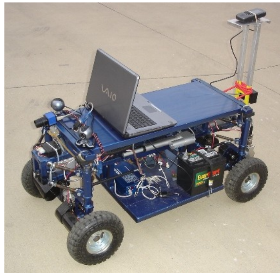
Figure 3: mini ODY-ERA (mOE), custom-made 1:3 scale autonomous vehicle.
