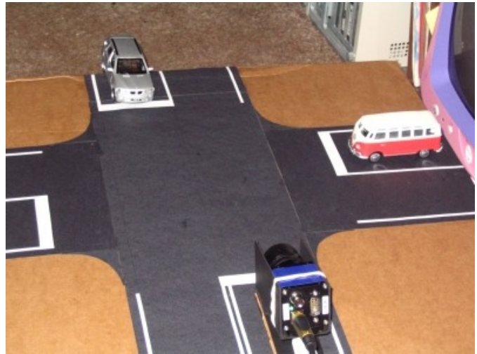
Figure 9: The 1:48 scale model of an intersection being utilized for algorithm verification purposes.
