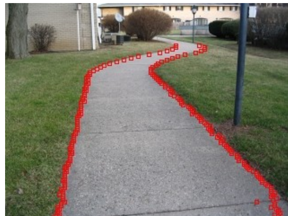
Figure 11: ‘Dots’ created by computing field gradients, as in Equation (4), followed by further processing to define the limits of the roadway.
