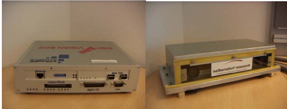
Figure 4. Embedded vision system (left) and external stereo sensor head (right)
