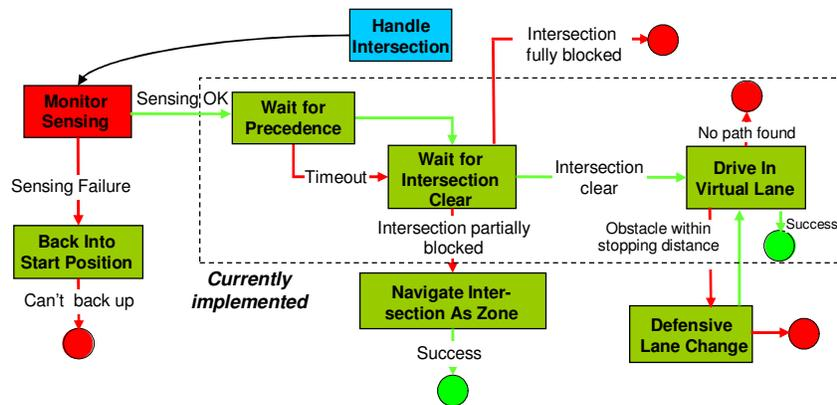
Figure 4. Schematic representation of the “Handle Intersection” behavior.
