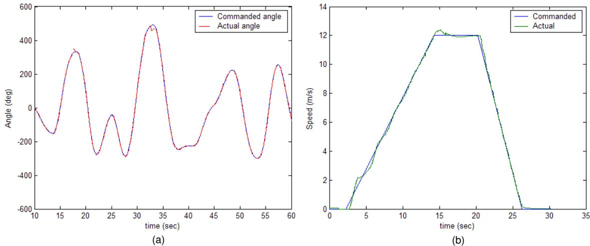
Figure 13. Representative steering angle and speed response curves.
