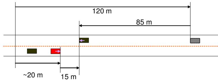
Figure 15. Passing a stopped vehicle with 30mph oncoming traffic requires a 120m sensing horizon for a stock Chevrolet Tahoe.
