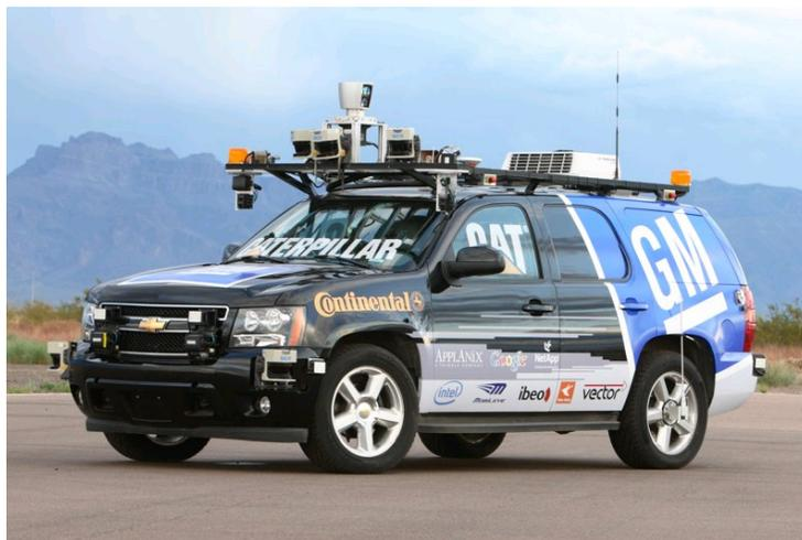
Figure 2. Boss, the Tartan Racing robot, is built on a Chevrolet Tahoe chassis. It incorporates a variety of lidar, radar and visual sensors to safely navigate urban environments.
