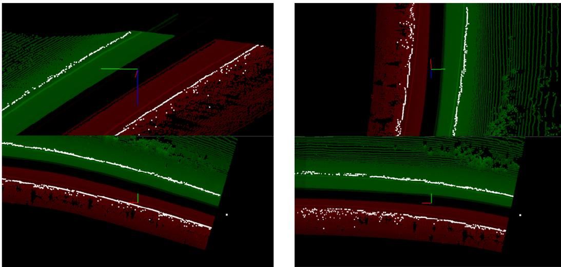
*Figure 12. Examples of the Haar road edge detection algorithm operating on stretches of straight and banked roads. Green and red dots show data from driver and passenger side looking SICK lasers. The detected road edge is marked white.*
