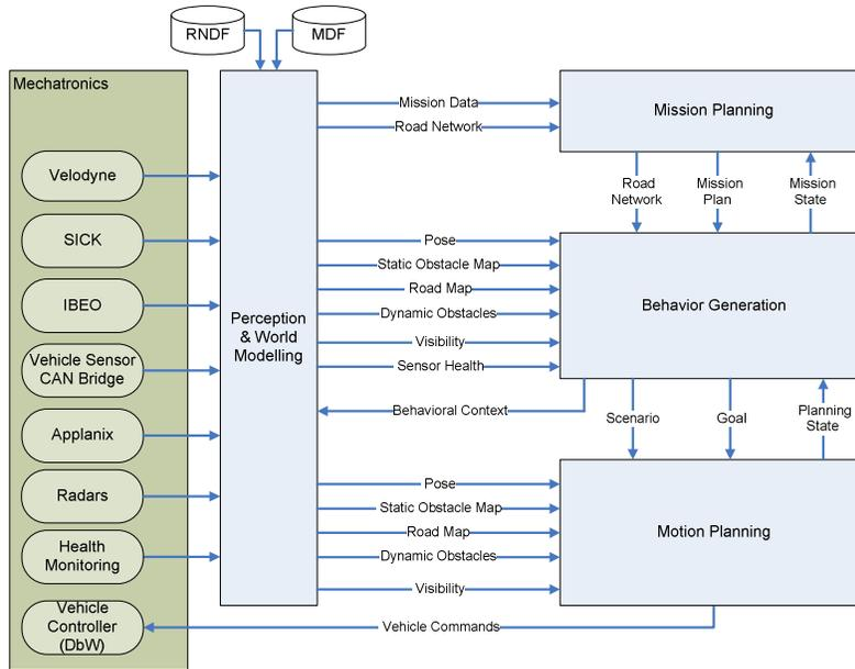
Figure 1. The Tartan Racing architecture is decomposed into five broad areas: Mission Planning, Motion Planning, Behavior Generation, Perception and World Modeling, and Mechatronics.
