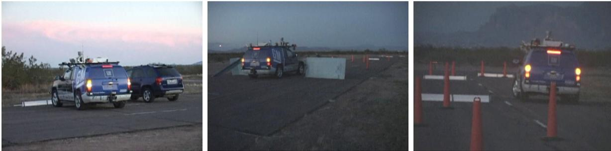
*Figure 16. The standard parking lot test includes a challenging obstacle field and a narrow opening. During system tests, the robot has successfully navigated this parking lot.*
