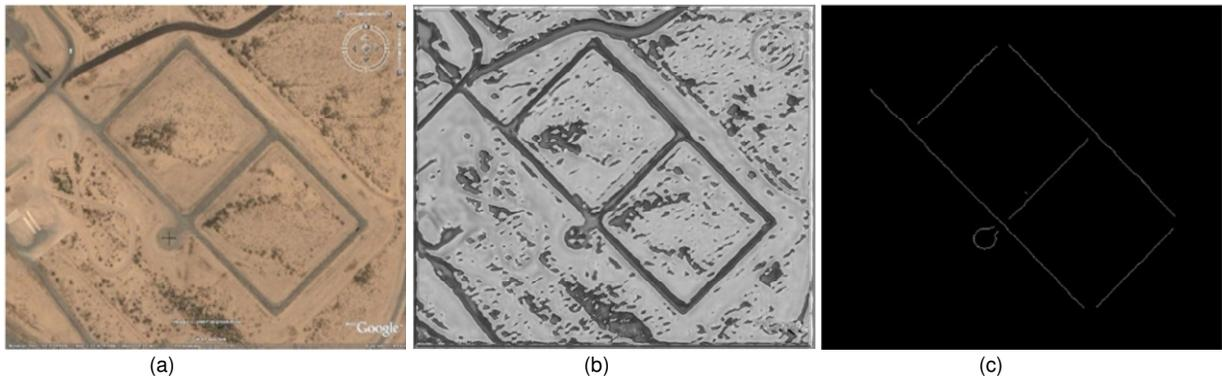
*Figure 11. Illustrates the off-line road shape extraction algorithm, (a) is an image of a road network, (b) shows the learned cost function and (c) shows the extracted road network.*
