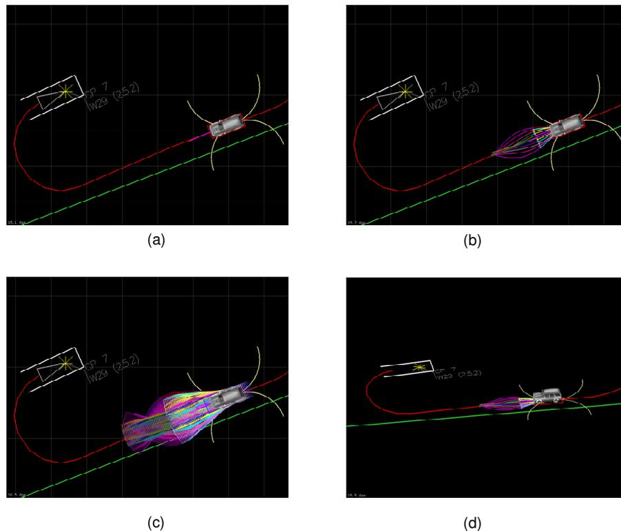
Figure 7. An illustration of the local planner following a lattice plan through a zone.
