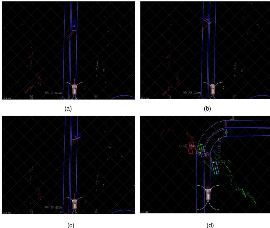
Figure 9. The moving obstacle fusion module following and tracking a vehicle as it performs a U-turn (a)-(c). The tracked vehicle is shown as a blue rectangle. In (d), a hard brake maneuver pitches the robot’s sensors down causing “ghost” objects to appear due to sensor reflections from the ground.
