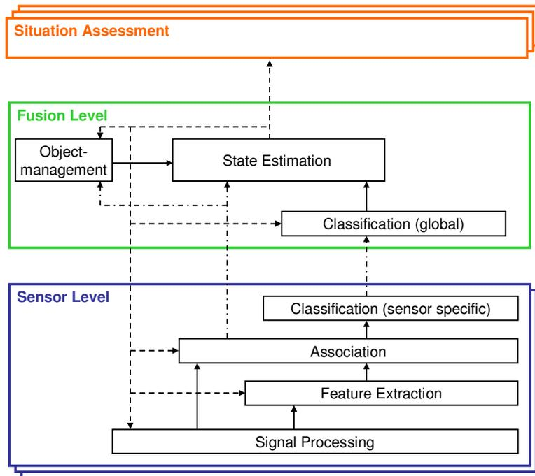
Figure 8. The moving obstacle fusion architecture supports multiple types of sensors.
