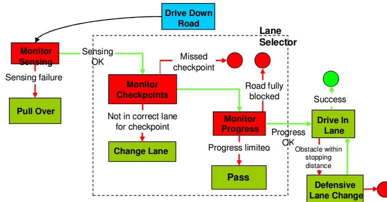
Figure 3. The Drive Down Road behavior. The Lane Selector portion is enclosed by dotted lines.
