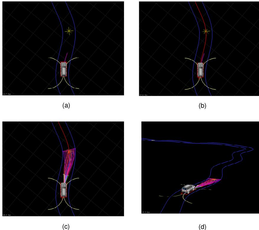
Figure 6. An illustration of the local planner following a road lane.
