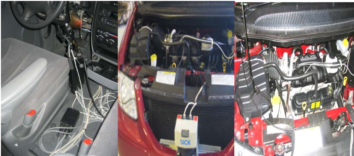
Figure 13. Implementation: drive-by-wire (left); SICK & controls (ctr); actuation (right)
