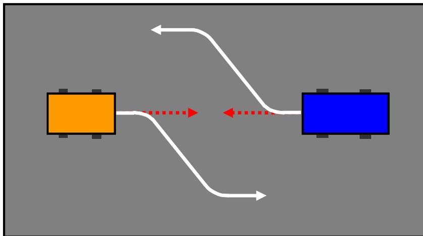
**Figure C.2** Two vehicles approaching head on in a zone. Collision is avoided by each vehicle staying to its respective right side.
