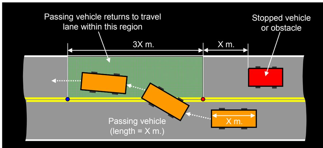
**Figure A.11** A vehicle completing a passing maneuver. The red dot marks one vehicle length from the front most point of the vehicle passed and the blue dot marks four vehicle lengths.
