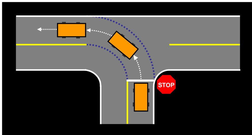
**Figure A.4** A vehicle making a left turn at an intersection. White dotted lines depict travel path through an intersection
