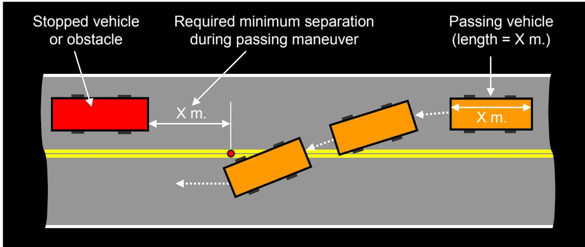
**Figure A.10** A vehicle initiating a passing maneuver. The passing maneuver must be completed without driving over the red dot that marks one vehicle length separation from the rear most point of the vehicle or obstacle.
