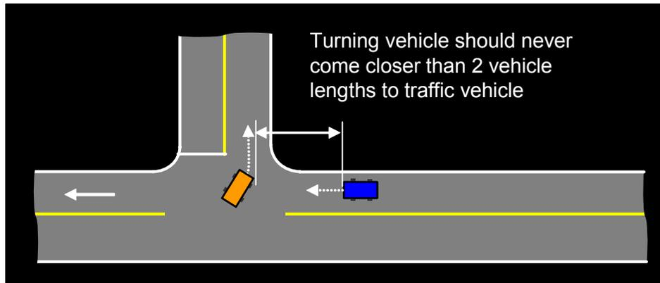
**Figure D.5** Safety standoff for left turn
