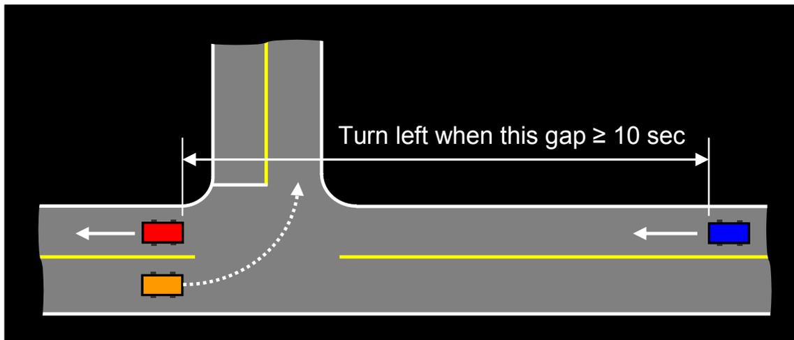
**Figure D.4** The orange vehicle must make the left turn across traffic when the indicated gap is greater than 10 seconds.
