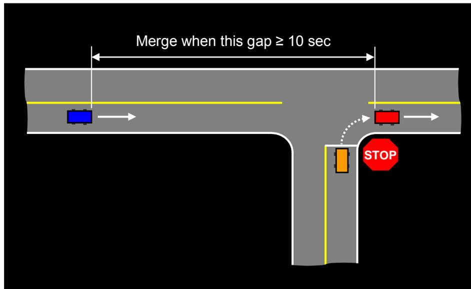
**Figure D.2** The orange vehicle must merge into traffic when the indicated gap is greater than 10 seconds.
