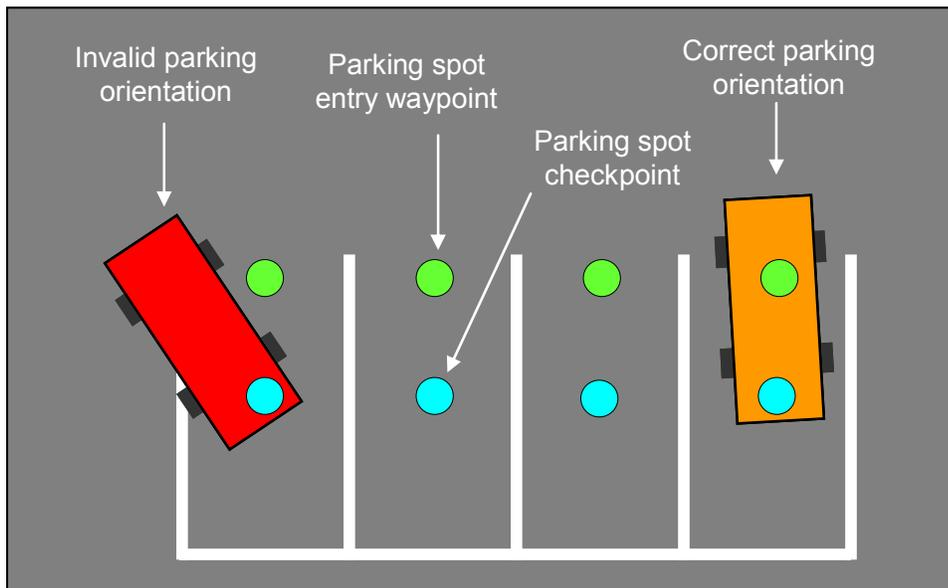
**Figure C.3b** Correct parking orientation
