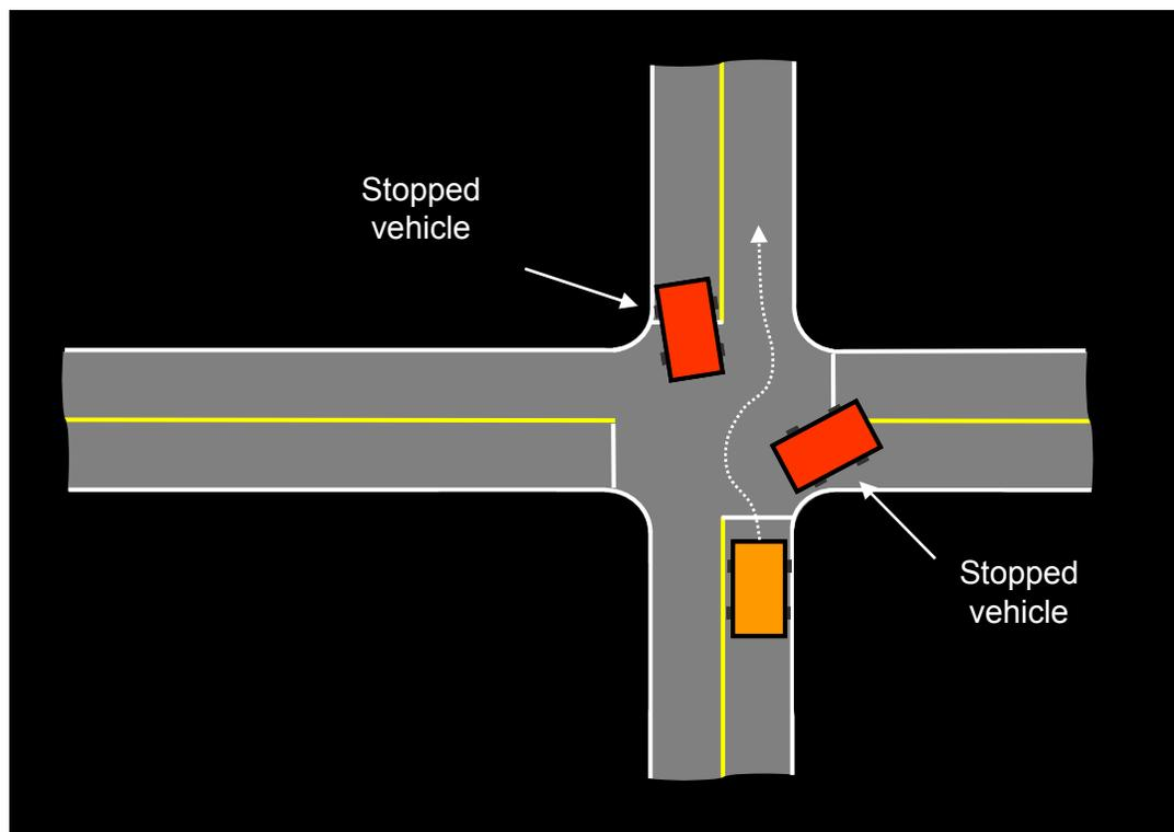
**Figure D.9** Stopped vehicles partially blocking an intersection
